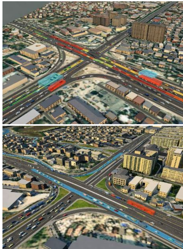
Figure 12. Traffic simulation and analysis at the junctions of Ish-Shqiponja interchange (left) and the Kombinat overpass (right). (source: Author, 2026).
