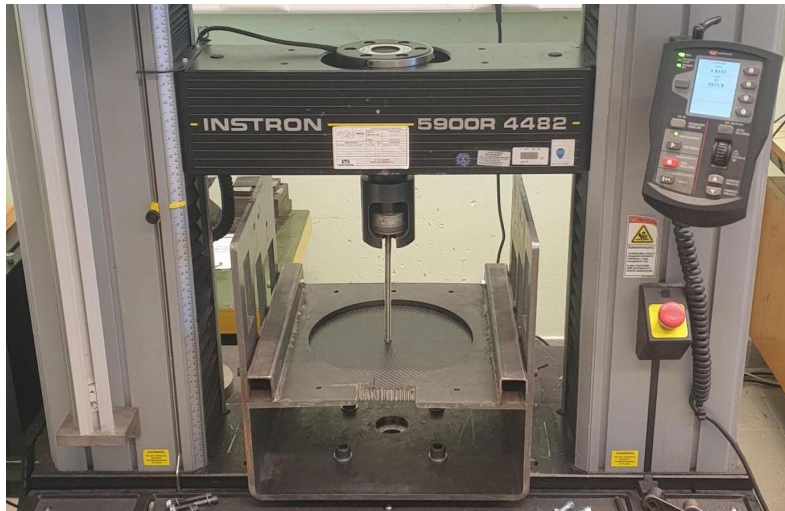
Figure 4. Test specimen in the clamping tool during empirical test.
