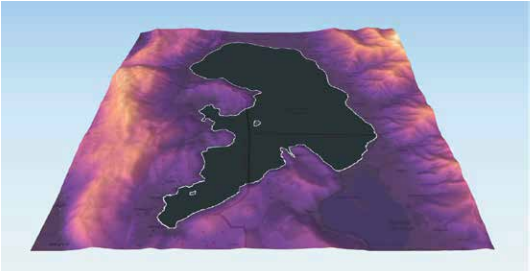
Fig. 4: The Great Prespa Lake 3D model from QGIS (through the qgis2threejs exporter plugin), with DEM + OSM derived texture.
