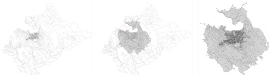
Figure 7 –a) Import all layers in the Grasshopper environment. b) Select only USUs inside a 10km radius area. c) Cull and restructure data branches accordingly. Elefront plugin was used for visualization.
