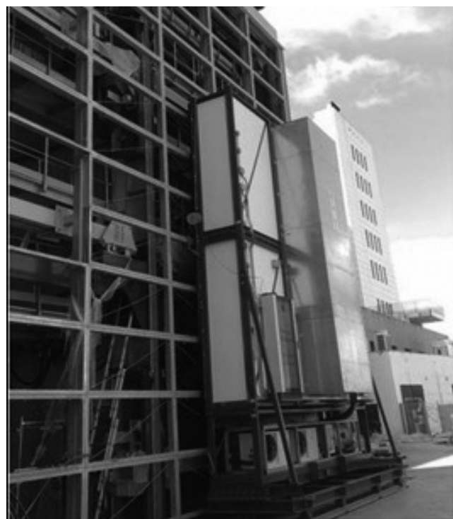
Figure 3. Fan capable of generating wind speeds equal to ~ 200 Km/h in accordance to the standard AAMA 501.1-05 “Standard Test Method For Water Penetration Of Windows, Curtain Walls And Doors Using Dynamic Pressure”, and all the other test with wind speed
