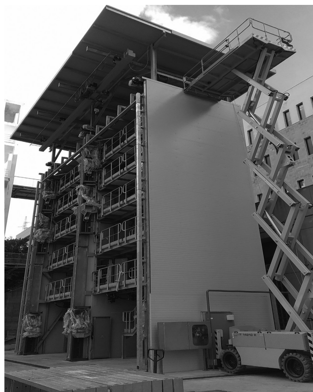
Figure 2. thermal Chamber, 15x12x4.5 m, or trying make-up with the AAMA 501.5-07
