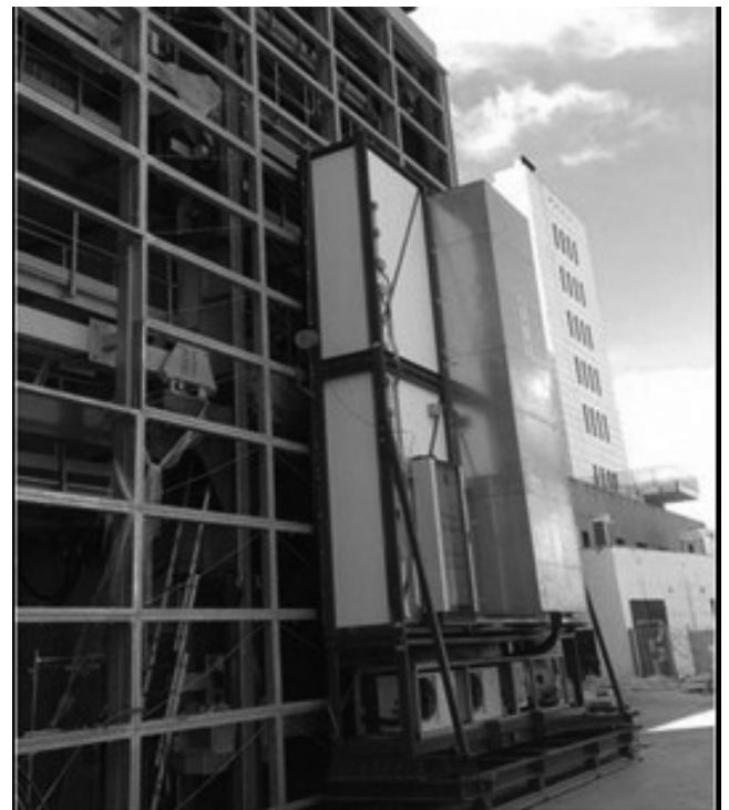
Figure 3. Fan capable of generating wind speeds equal to ~ 200 Km/h in according to the standard AAMA 501.1-05 “Standard Test Method For Water Penetration Of Windows, Curtain Walls And Doors Using Dynamic Pressure”, and all the other test with wind speed
