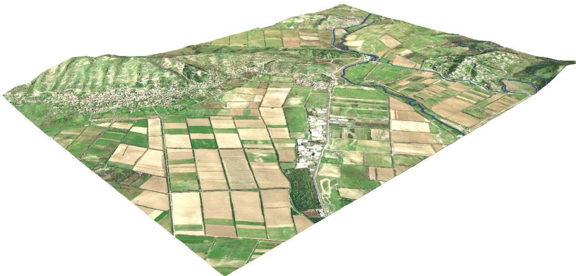
Fig8 / Infracore territorial model created by Model Builder tool, Bing data are overlaid on GIS data in order to create a realistic model with elevations and textures source / author
