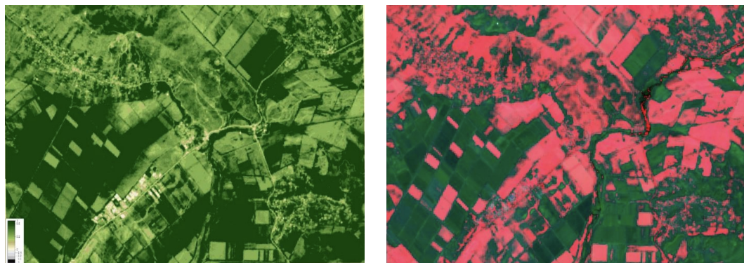
Fig5 / Remote Sensing analysis of vegetation and soil features from Sentinel Hub EO Browser, dataset Sentinel-2 L2A; (a) Normalized Difference Vegetation Index (NDVI) analysis; (b) Barren Soil Visualization analysis source / author
