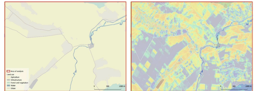
Fig6 / Comparison between land use and Remote Sensing analysis map; (a) Land use layer (National Agency of Territorial Planning, AKPT, 2021); (b) the overlay of the NDMI map on land use layer shows how within a single geometry there are different characterizations and data source / author
