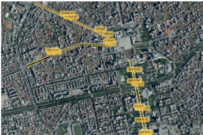
Fig.2/ The methodology of measuring the widths and lengths of the pavement Source/ Kelvi Peti using ASIG
