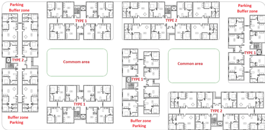
Fig. 2. Social housing proposed model; Type 1 – Studio and 1 BHK; Type 2 – 1 BHK and 2 BHK.
