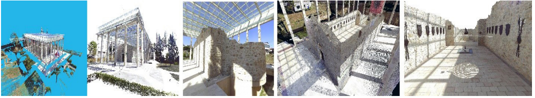
Fig.4/ The final point cloud, which contained around 110 million points. Source Diagram / Author
