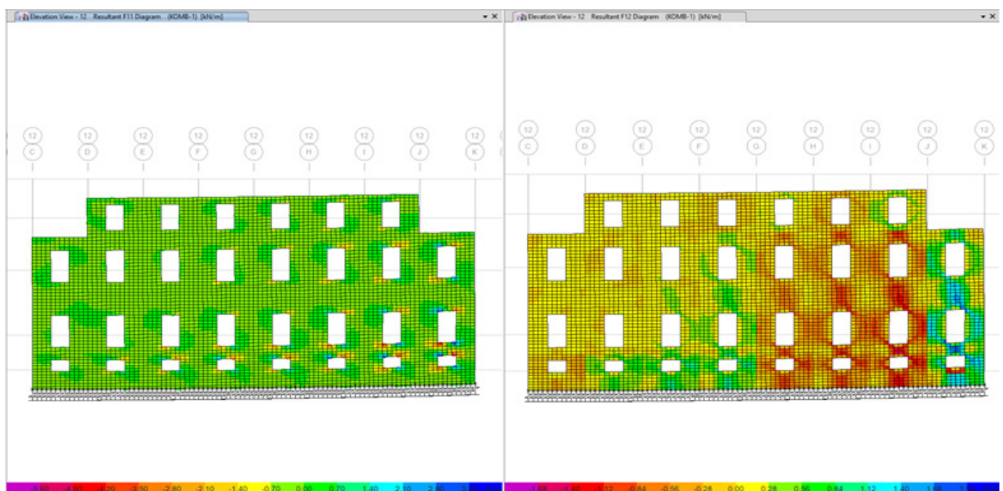
Fig. 8 Resultant Shell forces on main facade, f1-1 and f2-2 (ETABS, 2019)
