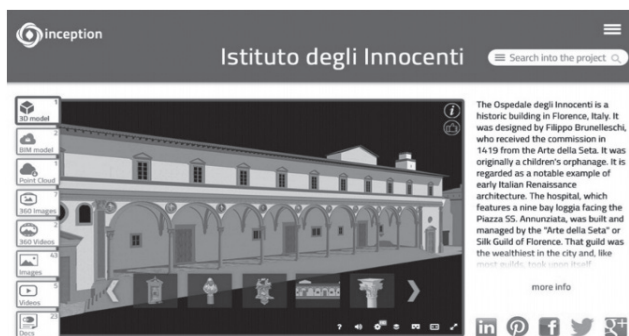
Figure 12. Inception Platform interface. 3D model and possible interactions (BIM model, point cloud, images, documents, videos, etc.) ( source: Maietti, F et al (2018)
