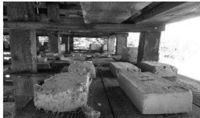
Figure 11. The different amount of straw inside the brick and its size, change the binding properties of the material and its finesse in appearance.
