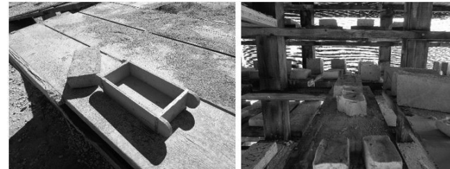
Figure 10. The table where the adobe material was placed and the mold made with wood, useful for the brick shape. In the right there are different shapes of adobe bricks
