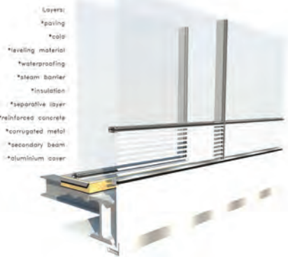
EXF Axonometric section of the facade
