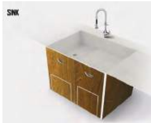
Fig.1 Sink Design Proposal adapted for washing the dishes while seating or with wheelchair
