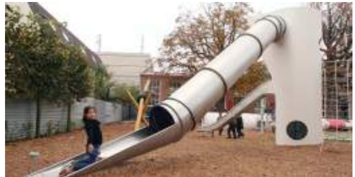
Wikado project 2012 Architects, playground made of recycled wind turbine blades (photo: Karola van Rooyen)
